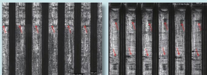
Figure 5: Manufacturing marks on the underside of different coloured staple strips in a box of SMK brand.
