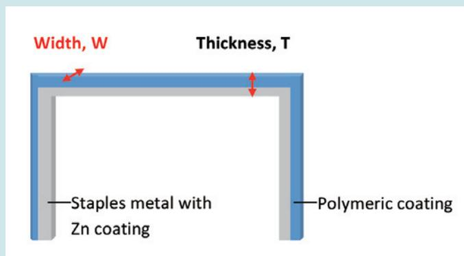
Figure 2: Width and thickness measurement
