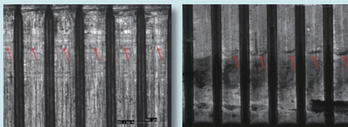
Figure 4: (Left) Manufacturing marks on the underside of coloured staple strips of DEL brand. (Right) Manufacturing marks on the underside of coloured staple strips of ETN brand.
