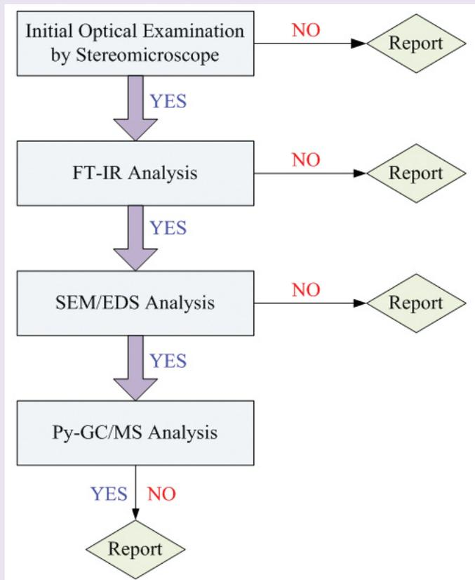
Figure 3: Flow chart showing proposed sequence for paint analysis
